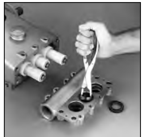
Removal of Lo-Pressure Seals
