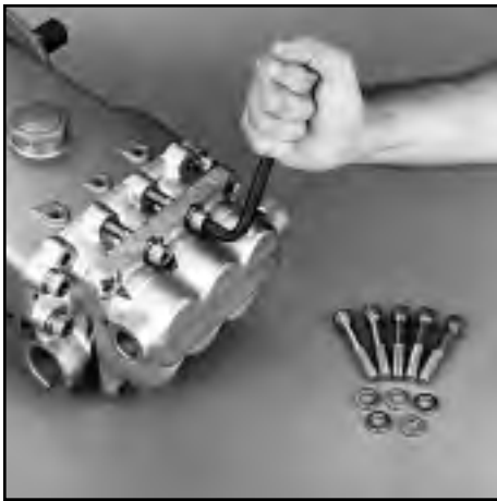
Removal of Discharge Socket Head Screws
