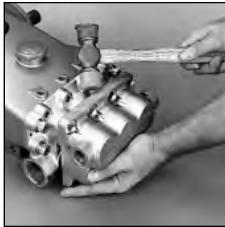
Separation of Discharge Manifold from Inlet Manifold
