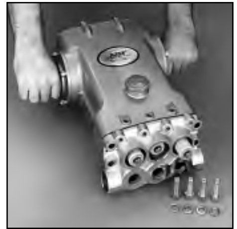
Rotate Crankshaft to position plungers
