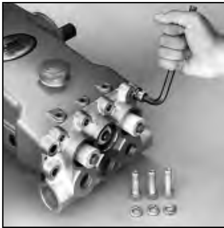
Removal of I.M. Socket Head Screws
