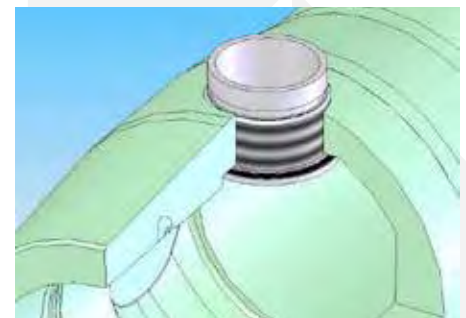
Seal seated against a flat surface
