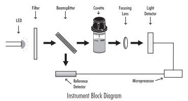
The internal reference system (reference detector) of the H197735 photometer compensates for any drifts due to power fluctuations or ambient temperature changes, providing a stable source of light for your blank (zero) measurement and sample measurement.
